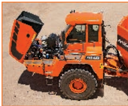
The hood has a wide opening (up to 83°) for easy access to the engine.
