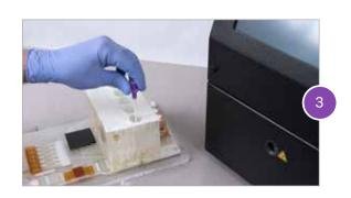
Insert sample into disposable chip
