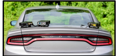
Figure 3: Trunk Mount 3Camera M7 System
