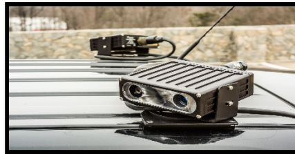
Figure 2: Roof Mounted M7 Camera
