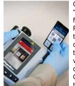
Choose "QuickDetect" from the main ResQ screen to activate the camera. Hold the pouch in view while centering the QR code within the yellow box.\*
