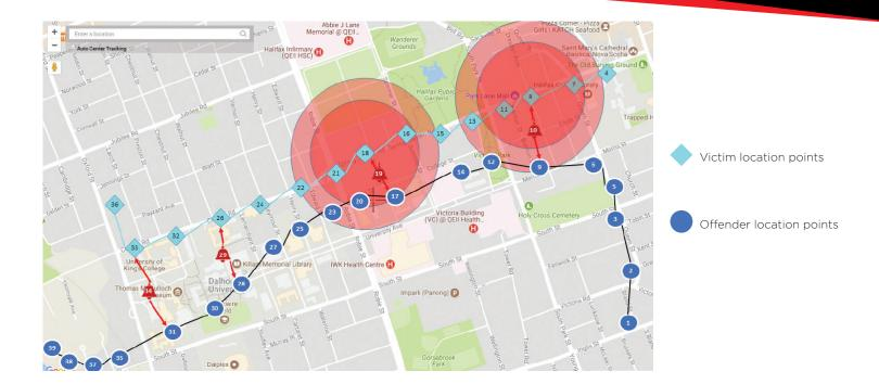
Once the app is installed, it communicates automatically with Track Group's system and syncs the smartphone with the offender's tracking device; activating the "mobile zone" created by officers. This zone moves with the smartphone and an alert is generated if the offender breaches the zone parameters.
