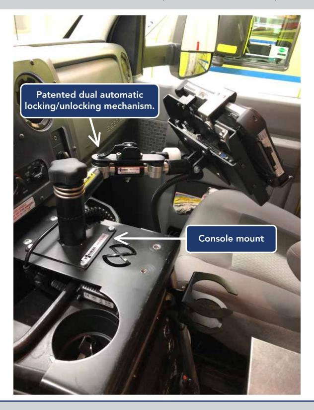
Any make / model of laptop, PC tablet or keyboard may be mounted to the Raca units.
