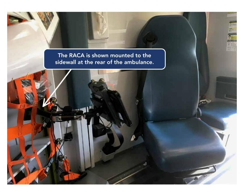
This was the only possible solution for this client, as a floor mounted mount would be obstrusive, and has no side console to mount the Raca.
